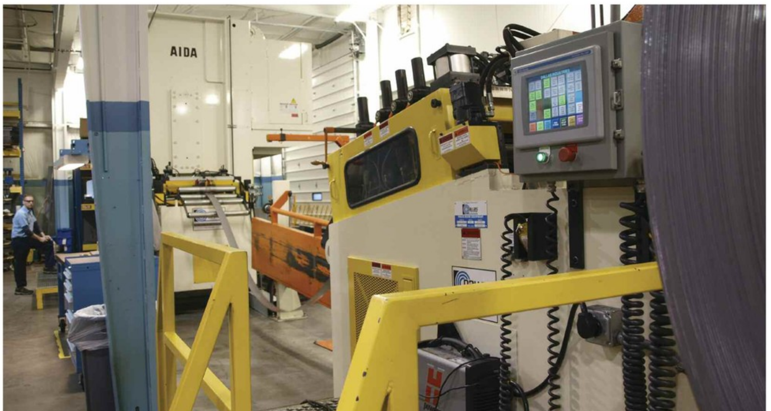
ATD outfitted its new coil line, which delivers material to a new servo press, with two complete and independent line-control stations, one at each end of the line. This saves operator steps and makes the setup process as efficient as possible.
