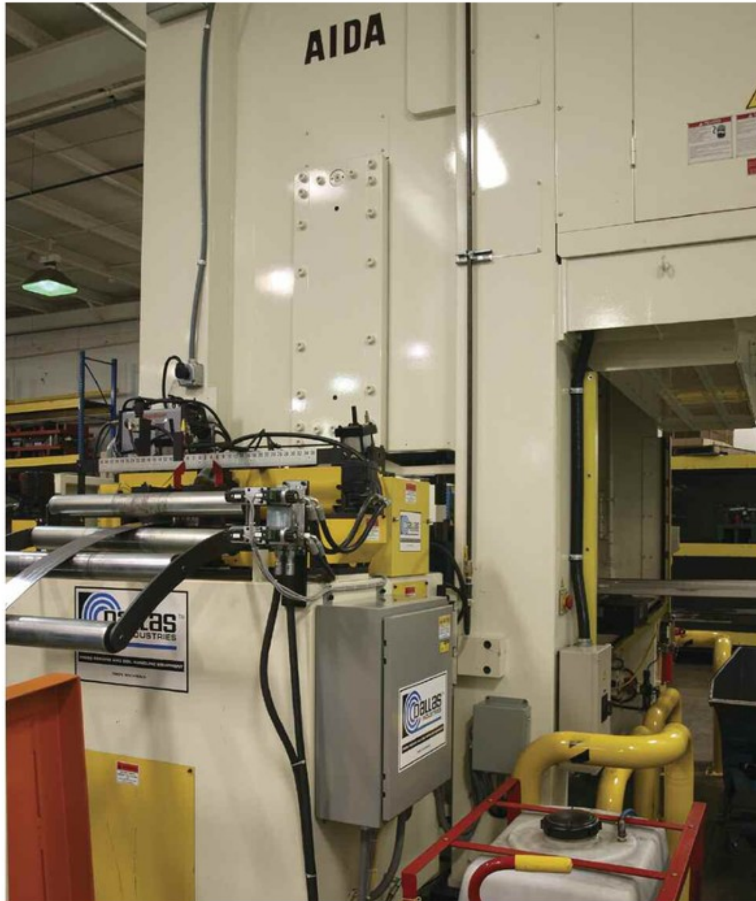
Noting that the feeder on its 600-ton press line has had some overheating issues when dealing with higher strength steels, ATD's Bennett says that the new line has the right gear ratio and motor capacity (20-hp motor with AC variable-frequency drive) to handle heavy-gauge high-strength work.
